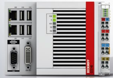
Embedded PC: IPC with integrated I/O level
